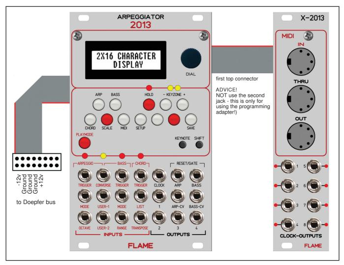
The module is delivered with a connected ribbon cable for the Doepfer bus. The red lead marks -12 volt. Connecting the module please note the right polarity!
