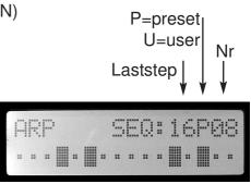
You can set also the sequence pattern with CV-inputs USER (see below Menu SETUP)
