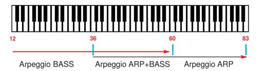
Splitzone for separatly / simultaneous playing of ARP- and BASS-Arpeggio
