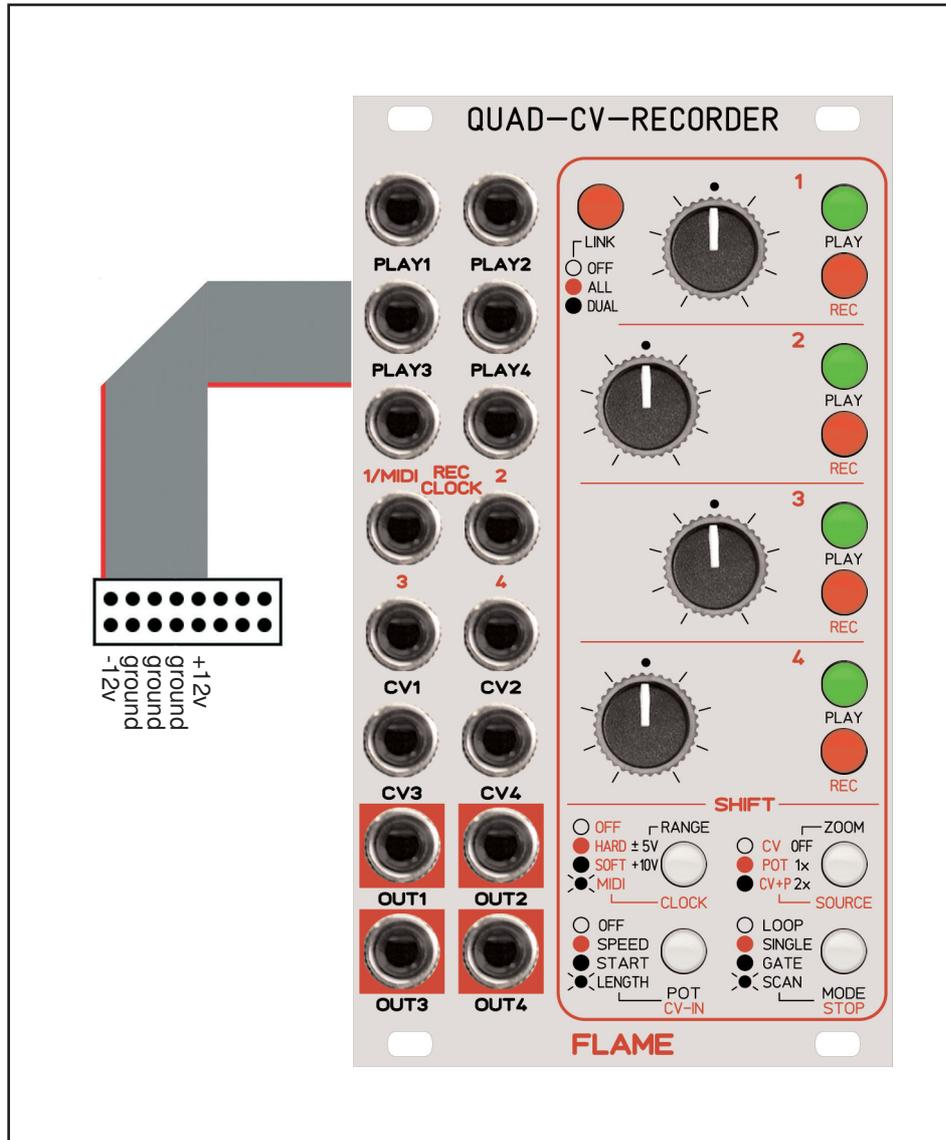
The module is delivered with a connected ribbon cable for the Doepfer bus. The red lead marks -12 volt. Connecting the module please note the right polarity!
