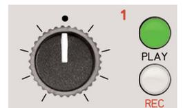
8. Stop the play back with buttons **SHIFT STOP + REC-1**. The output holds on the last sample voltage. If you turn the pot, then the output voltage switches to the voltage of the pot.
